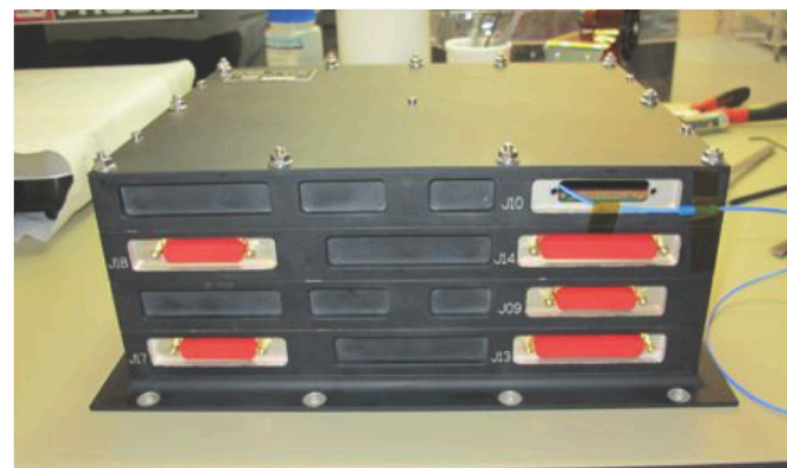
Unit assembled ready mechanical tests
